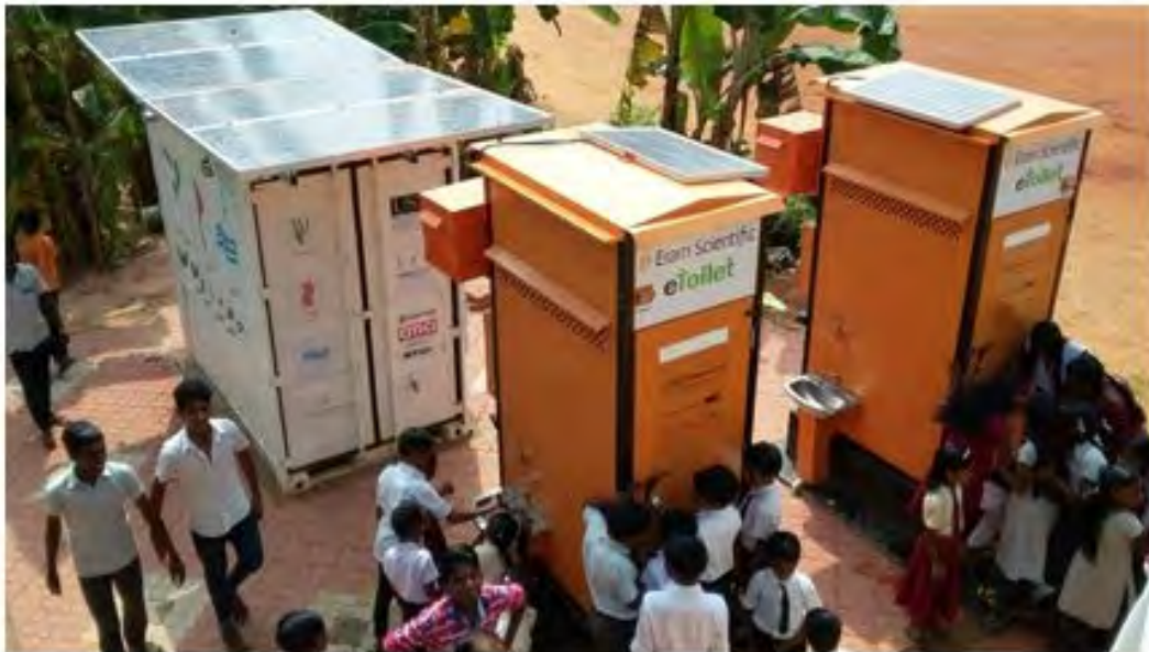
NEWgenerator 100 v.1 (white unit) Undergoing field-testing at a school in Kerala, India. The orange units are Earn eToilets serving as front-end units.
